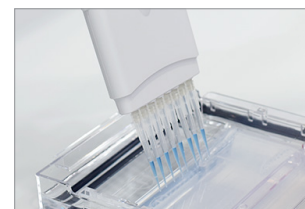
Multichannel pipettes can be used (31, 16 well combs)
